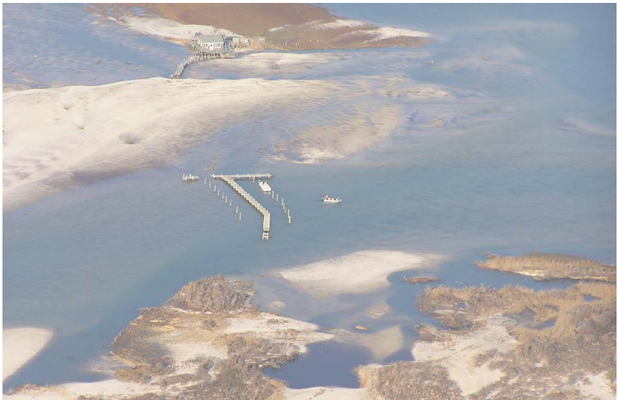
The new channel now passes under the old dock and connects the inlet to the old Old Inlet channel
